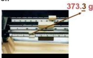
Uncertainty in measurements states we can estimate one past the lowest measurement. The number is halfway between 3.3 and 3.4, we record 3.35
